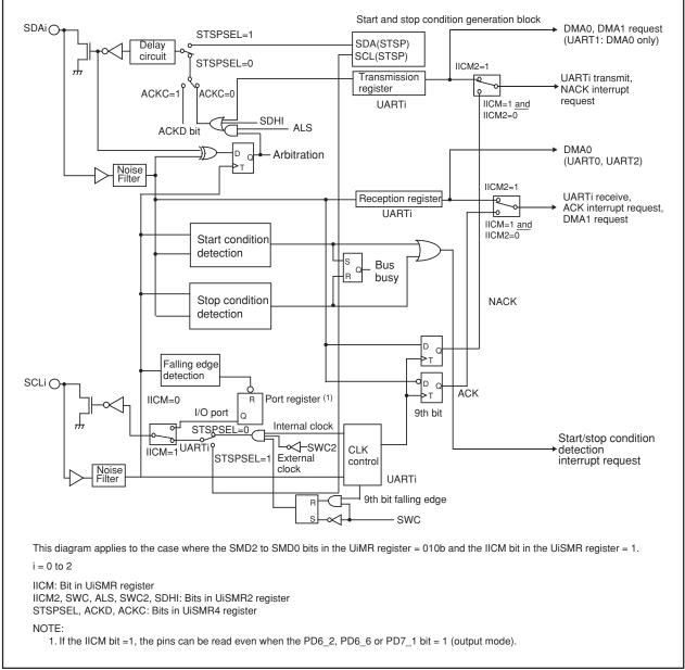
Figure 14.23 I<sup>2</sup>C Mode Block Diagram
